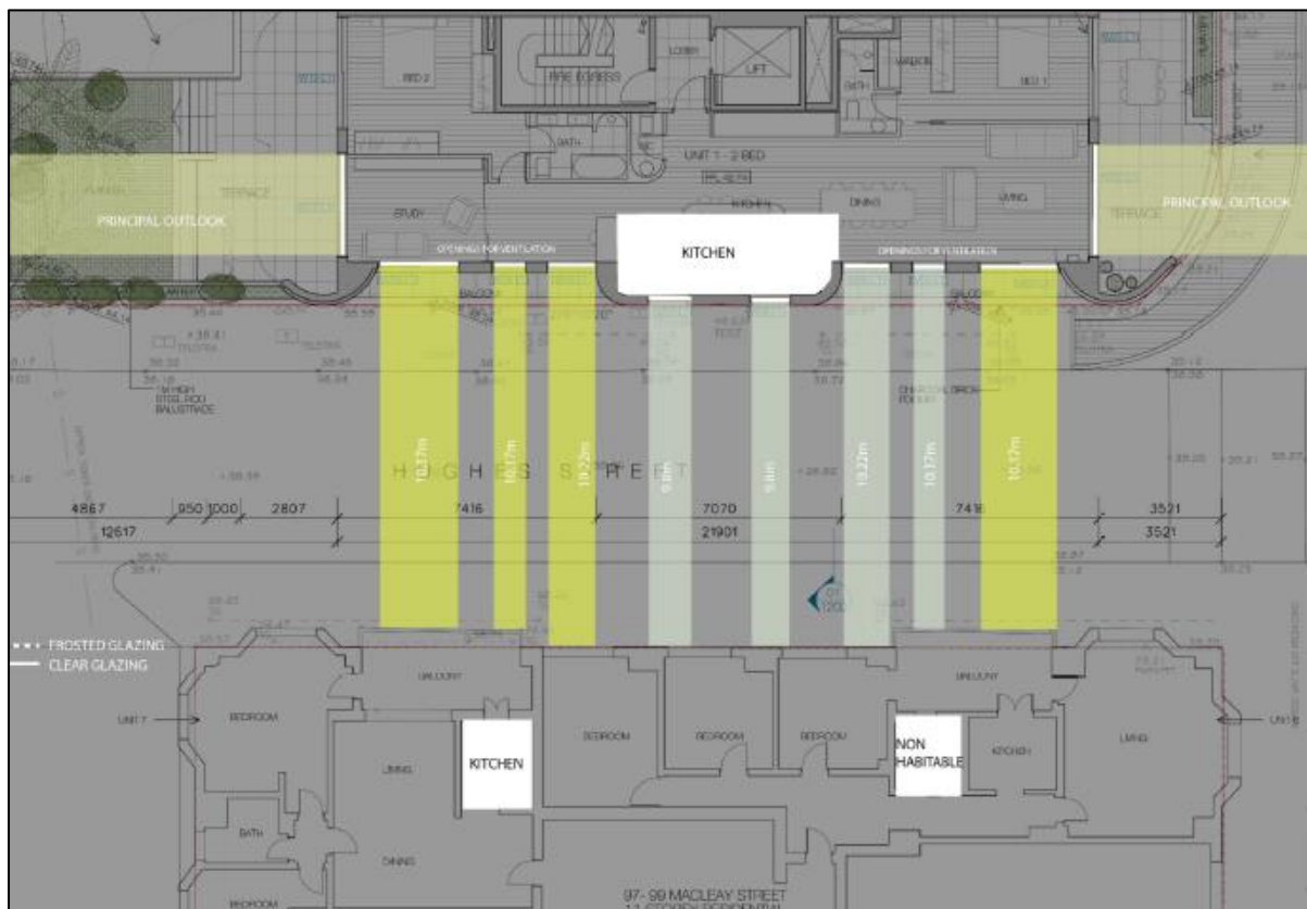
Figure 53: Privacy Diagram Ref: DA 2016 Rev F showing offset sensitive windows and balconies to remove direct lines of site to sensitive locations on Level 1
