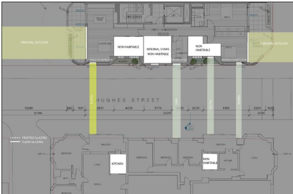
Figure 55: Privacy Diagram Ref: DA 2016 Rev F showing offset sensitive windows and balconies to remove direct lines of sight to sensitive locations on Level 4
